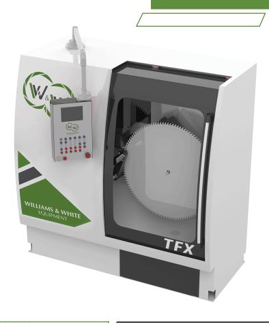
The Accusharp TFX Is a fully enclosed automatic top and face grinding machine for circular saw blades up to 36" (Optional 42") diameter. The automatic CNC operation allows the operator to continue his/her work as the machine sharpens the saws. Multi pass grinding and program saving make the TFx the ideal machine for any production or repair facility.
