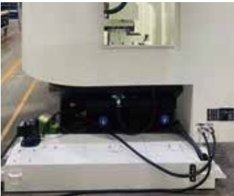
Coolant tank *Wet dressing
